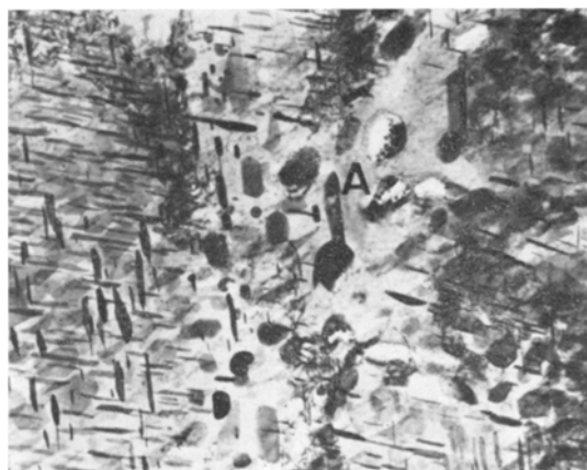
Figure 2 50% cold-rolled + 10 min 300° C. \gamma' precipitation and isometric \gamma crystals at "A" ( \times 20\,000 ).
